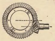
more "sliding" friction between the teeth compared with the spiral bevel "rolling" action. In order to prevent rapid wear of the expensive gear teeth a "powerful" type of extreme pressure oil must be used for hypoid rear axles, *i.e.*, Castrol HYPOY.
