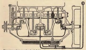
Here we see that every bearing is fed by oil under pressure, the big ends receiving their quota through passages drilled through the crankshaft, the oil entering these passages at the main crankshaft bearings. The surplus flung from the big end bearings lubricates the cylinder walls and little ends of the connecting rods, and then drains back to the sump.
