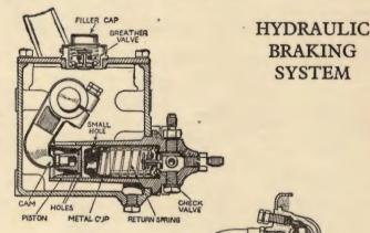
The Lockheed Hydraulic brake system is operated by means of oil pipe lines through which oil is forced under high pressure. This operates valves at each brake cam thus applying the brakes.
