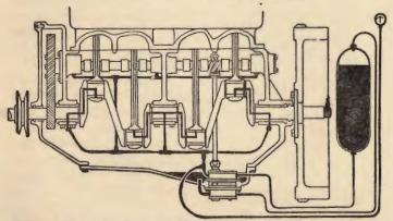
This is similar to the last system, with the exception that oil is pumped from a separate reservoir, and the sump is drained by a second pump, which returns the surplus oil to the reservoir. In this way a large body of oil is kept in circulation, which thus keeps cooler and remains cleaner for a longer period than a smaller quantity confined to the sump.
