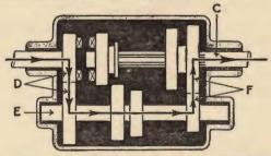
First or Low Gear.—Drive follows arrows through constant mesh pinions (d) to layshaft (e), and back through low gear pinions (f) to second motion shaft (c).
