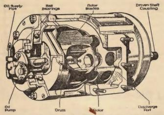
Lubrication connections for superchargers. Sectioned view of the Powerplus Supercharger. (Reproduced by courtesy of Powerplus (1927) Ltd.)
