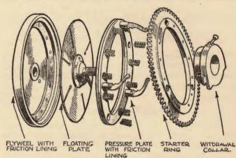
An "exploded" view of the Components of a single plate clutch. (By courtesy of "The Light Car and Cycle-car.")
