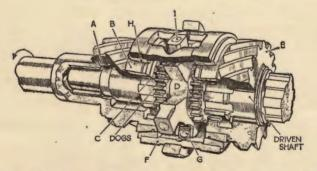
This type of gear enables the speed of two dogs to be synchronised automatically as they are pressed into engagement by the gear lever.
