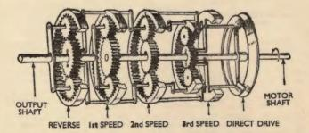
The principle of the WILSON GEAR BOX. When the brake band closes on any one of the drums illustrated and prevents it rotating the Planet wheels must rotate inside the stationary drum and that gear is then in engagement.
