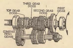
A type of gear box with three sets of constant mesh pinions, or "silent" third and second gears. In top gear, of course, the power is transmitted direct through the main shaft. (By courtesy of "The Autocor.")
