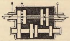
Fourth or Top Gear.—Drive follows arrows direct from engine through dogclutch (a), connecting first (b) and second (c) motion shafts to rear axie.
