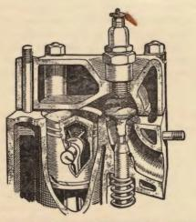
This illustration shows how in course of time carbon forms inside the combustion chamber, on the piston top, inside the piston, and on the valve head.
