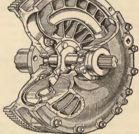
The diagram above illustrates the principle upon which the Hydraulic Clutch of "Fluid Flywheel" operates. Below is a sectional drawing of the actual mechanism showing the simplicity of its construction. (By courtesy of "The Autocar.")
